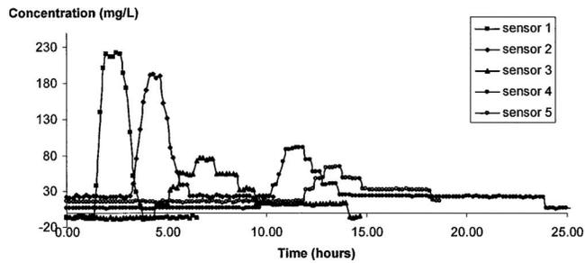
**Fig. 4.** Combined breakthrough curves for Sensors 1–5 with calibrated values
