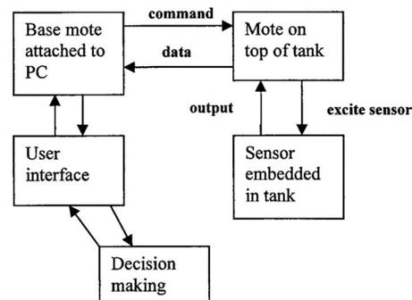
Fig. 3. Schematic of the wireless sensing communication system
