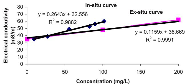
Fig. 12. In situ and ex situ calibration curves for Sensor 1
