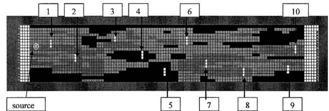
**Fig. 5.** Final sand distribution model after tank packing and sensor placement
