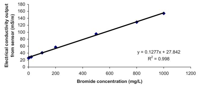
**Fig. 1.** Calibration curve for Sensor 1 in solution
