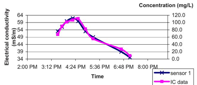
**Fig. 6.** Breakthrough curve for Sensor 1 with IC data
