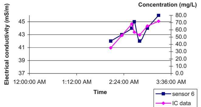
Fig. 10. Selected points from the breakthrough curve for Sensor 6 compared to IC data
