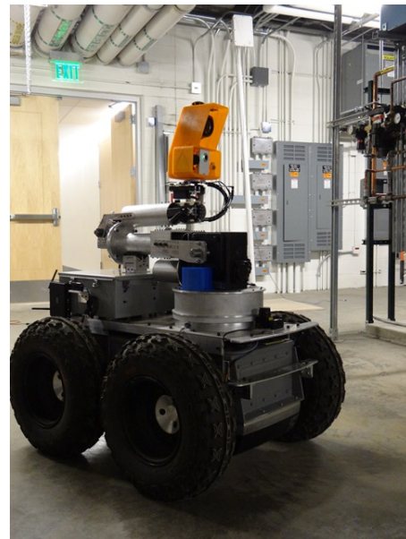
Fig. 1. A refinery inspection mobile robot
