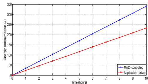
**Figure 8:** Energy consumption comparison between Application-driven and MAC-driven antenna state transition methods in arrangement-1
