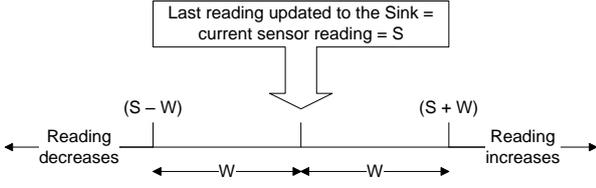
**Figure 2:** The value of a sensor node right after an update
