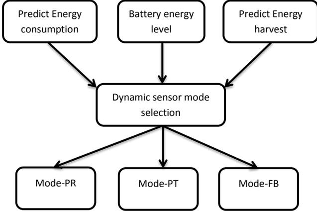
**Figure 3:** Application-driven mode transition (MAC-driven variant has only two modes)
