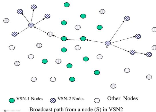
Figure 1: An example of two VSNs over the same physical sensor network infrastructure.
