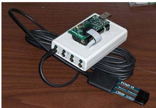
Fig. 2. A TelosB mote is attached to a ECH<sub>2</sub>O probe through a breakout box.
