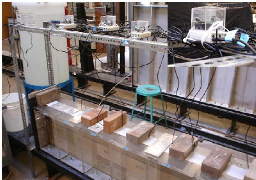
Fig. 5. Tank testbed. The motes are placed on top of the tank, attached to a rack.
