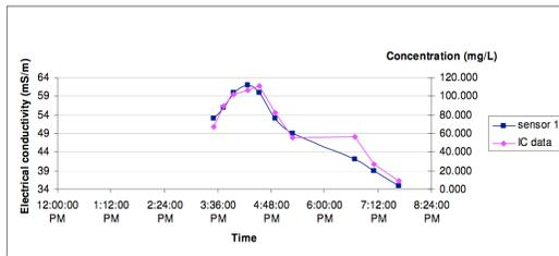
**Figure 3. Electronic conductivity and concentration values of sensor 1**
