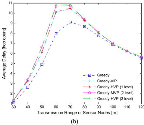
Fig. 6. Average delay of the Greedy algorithms with different communication ranges
