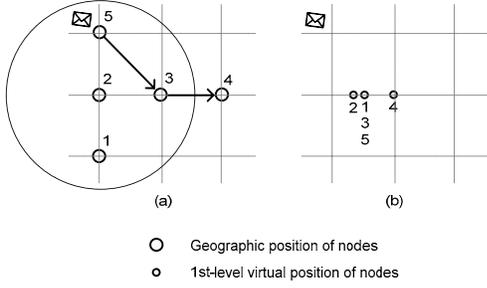
Fig. 4. An example of routing holes introduced by using virtual positions.
