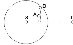
Fig. 1. An example of Greedy and MFR geographical routing. A packet is sent from node S to node D. The Greedy algorithm selects node A as the next-hop, since A is the neighbor that is the closest to the destination. The MFR algorithm selects node B as the next hop, since B makes the greatest progress along the direction of packet forwarding (S-D). Both Greedy and MFR requires the next hop to be closer to the destination than the current node.
