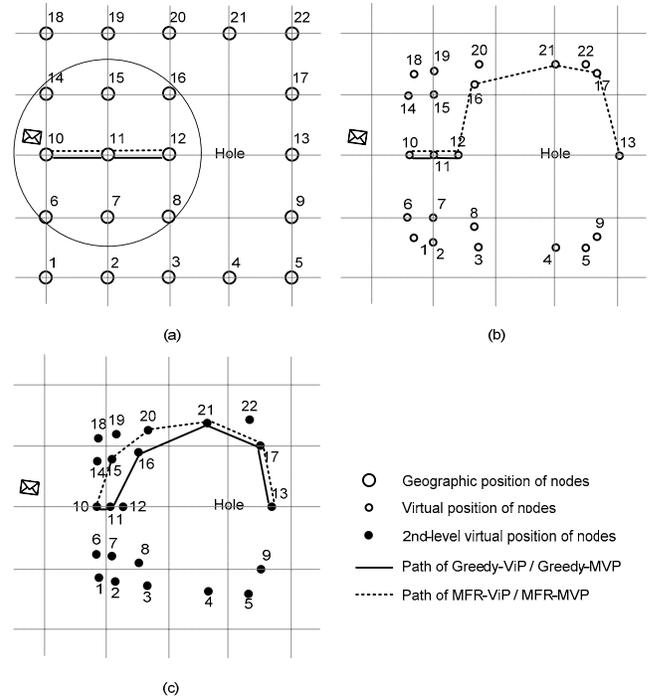
Fig. 3. An example of using virtual positions in GF. The packet is routed from node 10 to node 13. When using the geographic positions of nodes, node 12 becomes a local minimum for both Greedy and MFR, as shown in (a). With virtual positions, a path can be found by MFR-ViP, as shown in (b). With 2<sup>nd</sup>-level virtual position, both Greedy-MVP (2-level) and MFR-MVP (2-level) find paths around the hole, as shown in (c).
